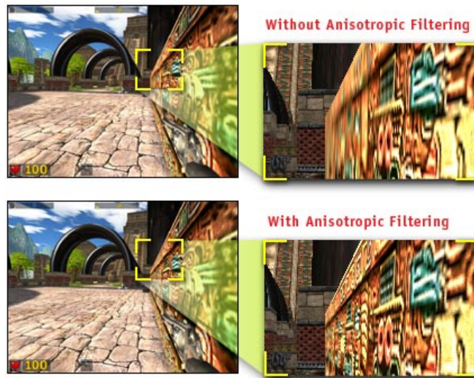
Figure 1. This wall, from a scene in Serious Sam: The Second Encounter , illustrates the dramatic effect that anisotropic filtering can have on image quality.
